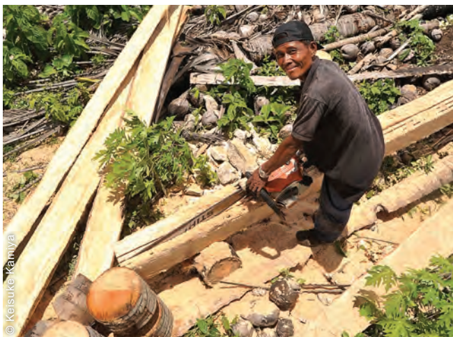
Local people cut fallen coconut trees into planks with chainsaws (Guiuan).
