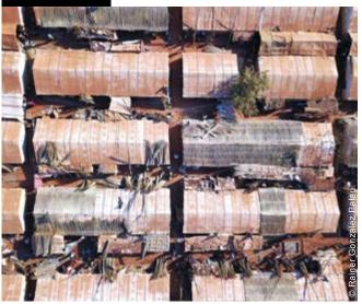
One of the upgrades consisted of adding a layer of dry elephant grass to rooftops to increase protection from the elements, improve ventilation and lower inside temperatures.
