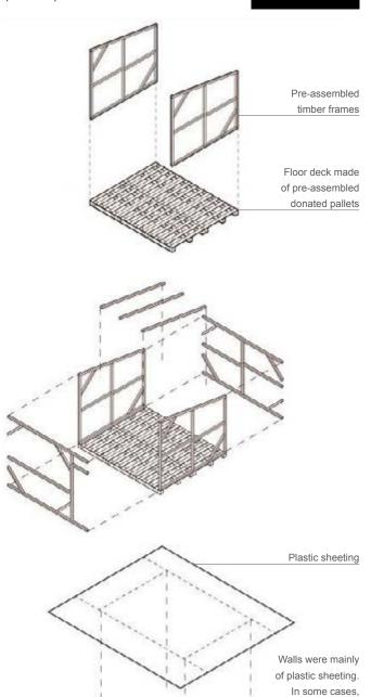
The shelter had a self-build design, with wooden structure and plastic walls. The construction changed over time, depending on the materials available (image source: Help Refugees).
