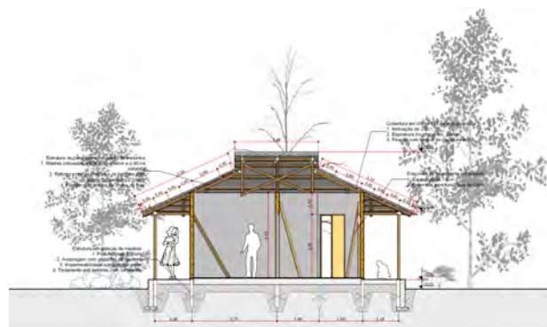
Longitudinal section of the 2-bedroom model house.
